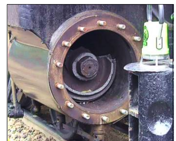
Photo: Olaf Rasmussen Cylinder head removed shows damaged piston
