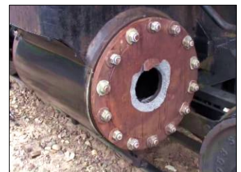
Photo: Olaf Rasmussen Damage to the cylinder head halted the engine
