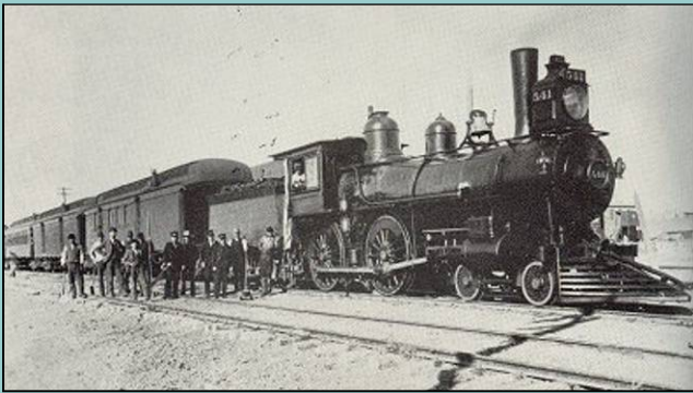
Photo: Kansas City Historical Society The standard engine in AT&SF freight service from 1880–1910 was the 4-4-0 type engine
